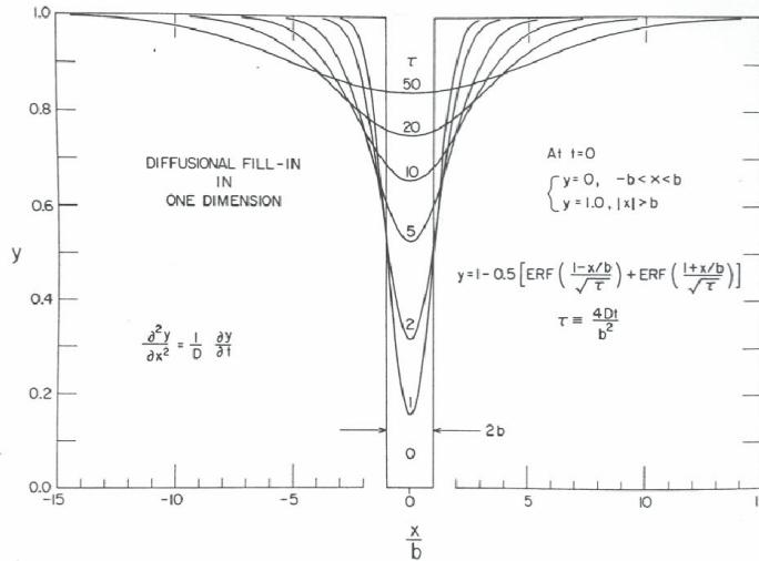
Fig. 23. A family of calculated curves illustrating the time dependence of the one-dimensional diffusive fill-in of the charged particle shadow of a satellite of radius  $b$  for particles whose radius of curvature is much less than  $b$  (Van Allen et al. 1980b).
