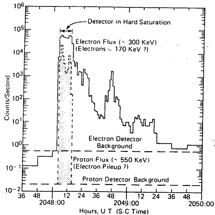
Fig. 1. The B event during Mercury encounter, adapted from *Simpson et al.* [1974a]. The labels 'electron flux ( $\sim 300$  keV)' and 'proton flux ( $\sim 550$  keV)' are those of *Simpson et al.* [1974a]. All other labels have been added, with the exception of the label on the time axis.
